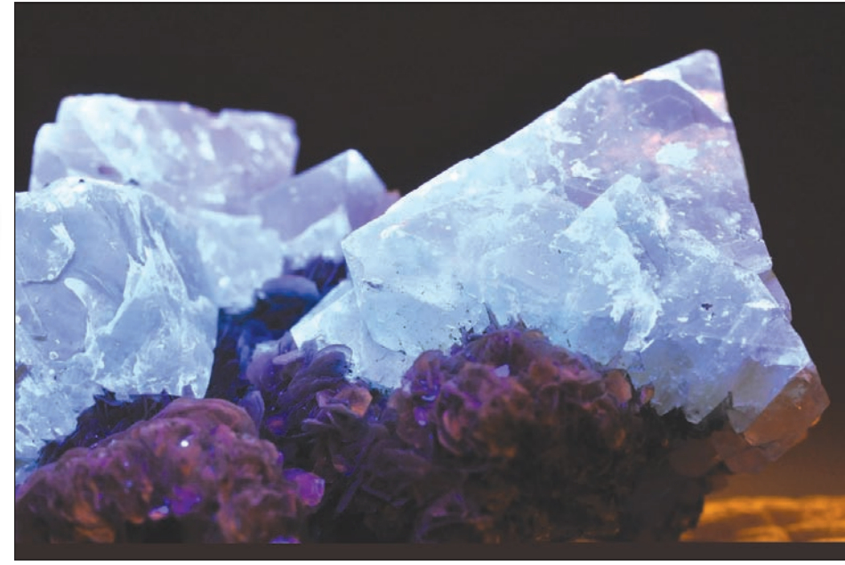
Scheelite crystals and muscovite mica showing fluorescence under ultraviolet radiation. Image courtesy of Commons Wikimedia: image released to public domain.
